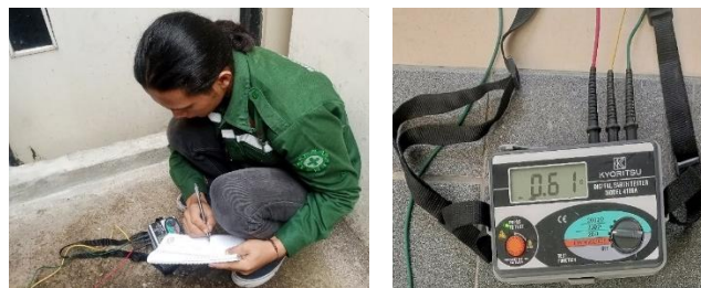
Figure 4. Measuring Soil Resistivity with Earth Tester
